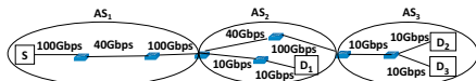
Figure 2: An example where a user wants to reserve bandwidth for three source-destination pairs: (S, D_1) , (S, D_2) and (S, D_3) .
